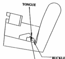
Note: THE SEAT BELT WEBBING MUST CONTACT THE CURVED EDGE ON BOTH SIDES OF THE FIXTURE
