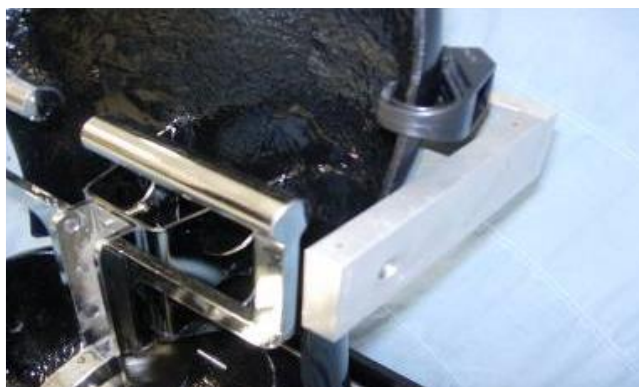
Figure 17: H-PM back pan held by retaining strap.
